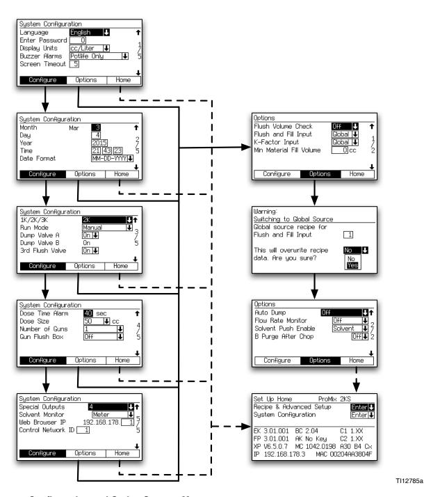
Fig. 21. System Configuration and Option Screens Map
